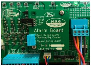
3. Adjust volume of the buzzer using the J3 jumper. Jumpering Pins 1 to 2 provides the loudest setting, Pins 2 to 3 the softest setting and Pins 3 to 4 are for off.
