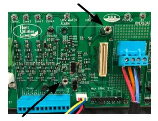
2. Mount the alarm on the stand-offs re-using the 2 screws.
