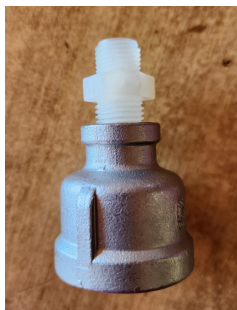
3/4" to 1/4" stainless steel adapter with nylon fitting
