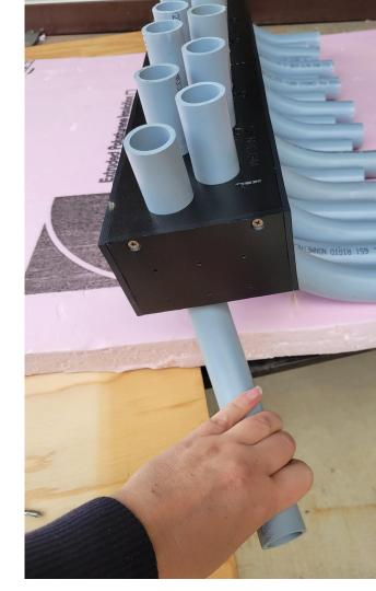
4. Slide the H4 over the stakes, so the stakes are at the back of the H4. Secure the H4 with short screws through the predrilled holes in the H4 wall.
