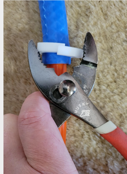
Squeeze sides of clamps together with slip joint pliers in wide mode.
