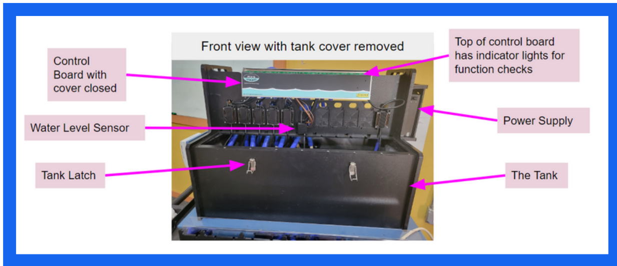
Graphic 1) Front View with Tank Cover Removed
