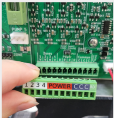
The 12 pin wire connector gently pulled off the control board.
