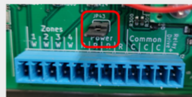
Jumper #JP43 is circled in red. Remove it when powering a smart thermostat.
